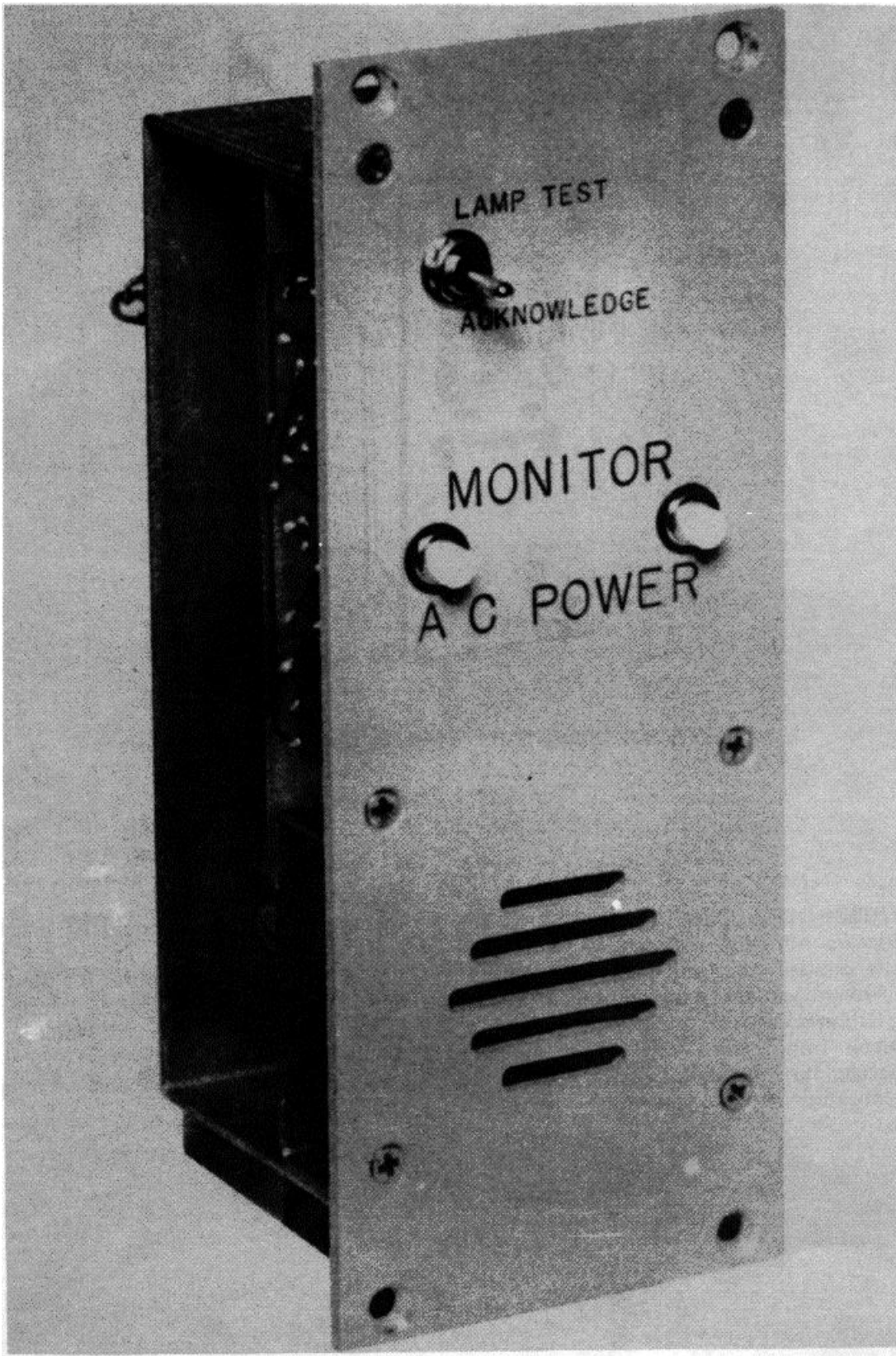
Figure 3-2. Monitor Cabinet (Signal Module) Controls and Indicators
